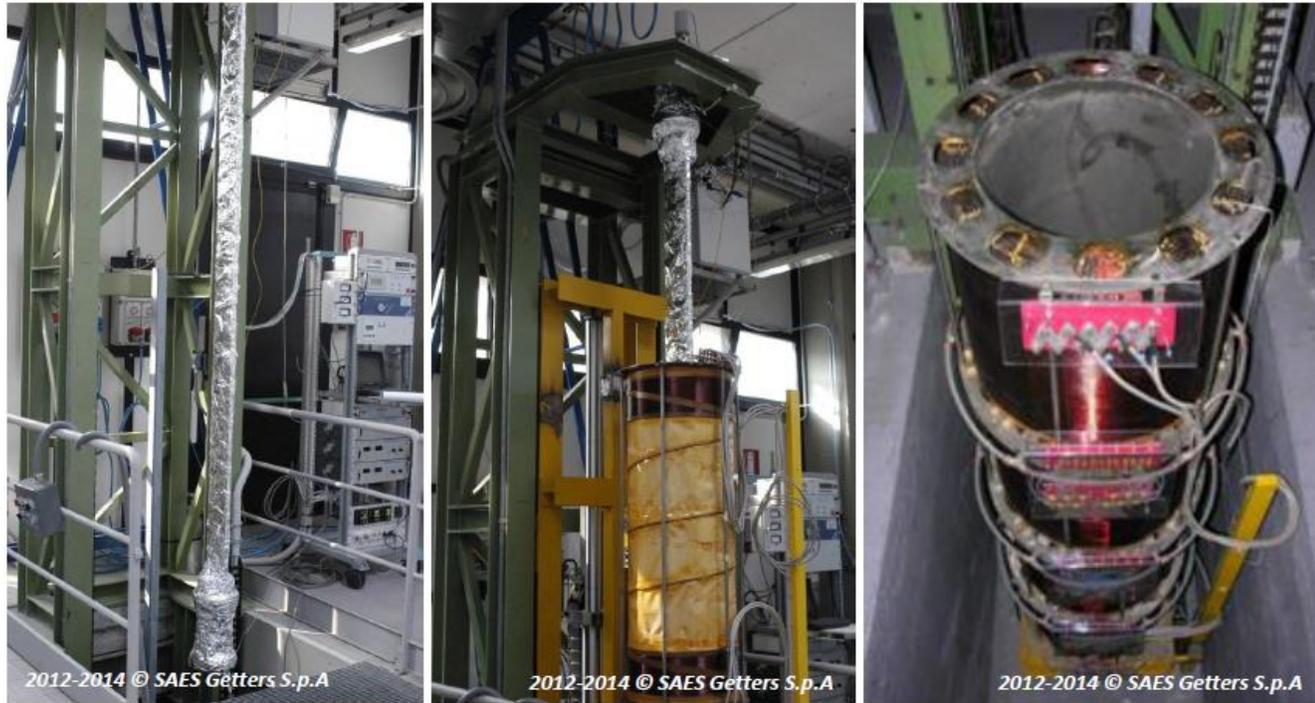
One of the SAES sputtering systems for NEG coating, capable to coat up to **6.5 meter** long chambers with a **2m** height coil.
